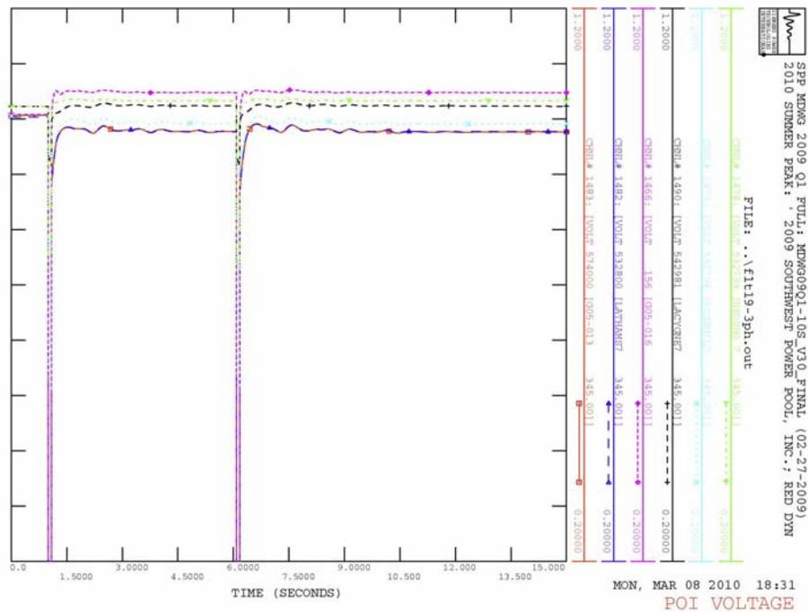
Figure 4-2. POI Voltage Plot for Fault 19 – FERC 661A Fault; 3-Phase Fault on the GEN-2005-013 to GEN-2005-016 345 kV line, near GEN-2005-013
