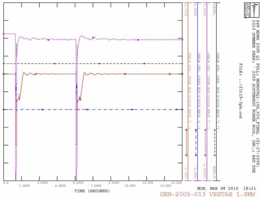
Figure 4-1. GEN-2005-013 Plot for Fault 19 – FERC 661A Fault; 3-Phase Fault on the GEN-2005-013 to GEN-2005-016 345 kV line, near GEN-2005-013
