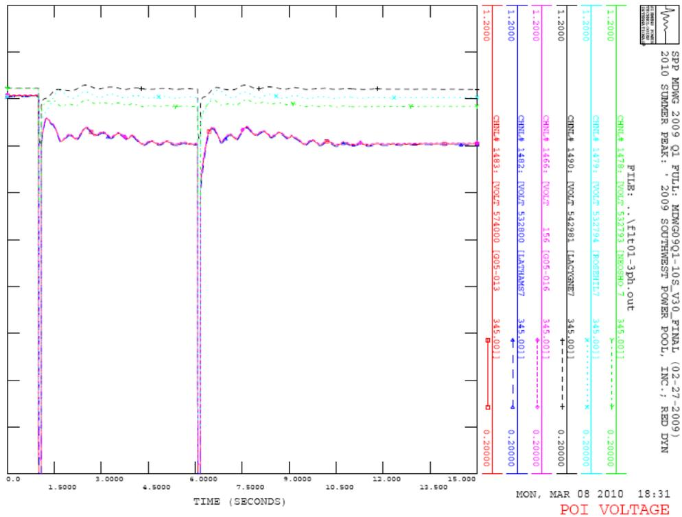
**Figure 4-4. Local 345kV Buses Voltages Plot for Fault 1 – 3-Phase Fault on the Rose Hill to the Latham Switching Station 345kV Line, at Mid Line**
