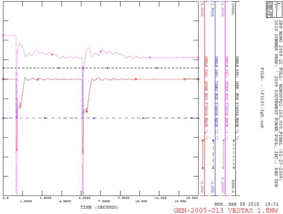
**Figure 4-3. GEN-2005-013 Plot for Fault 1 – 3-Phase Fault on the Rose Hill to the Latham Switching Station 345kV Line, at Mid Line**
