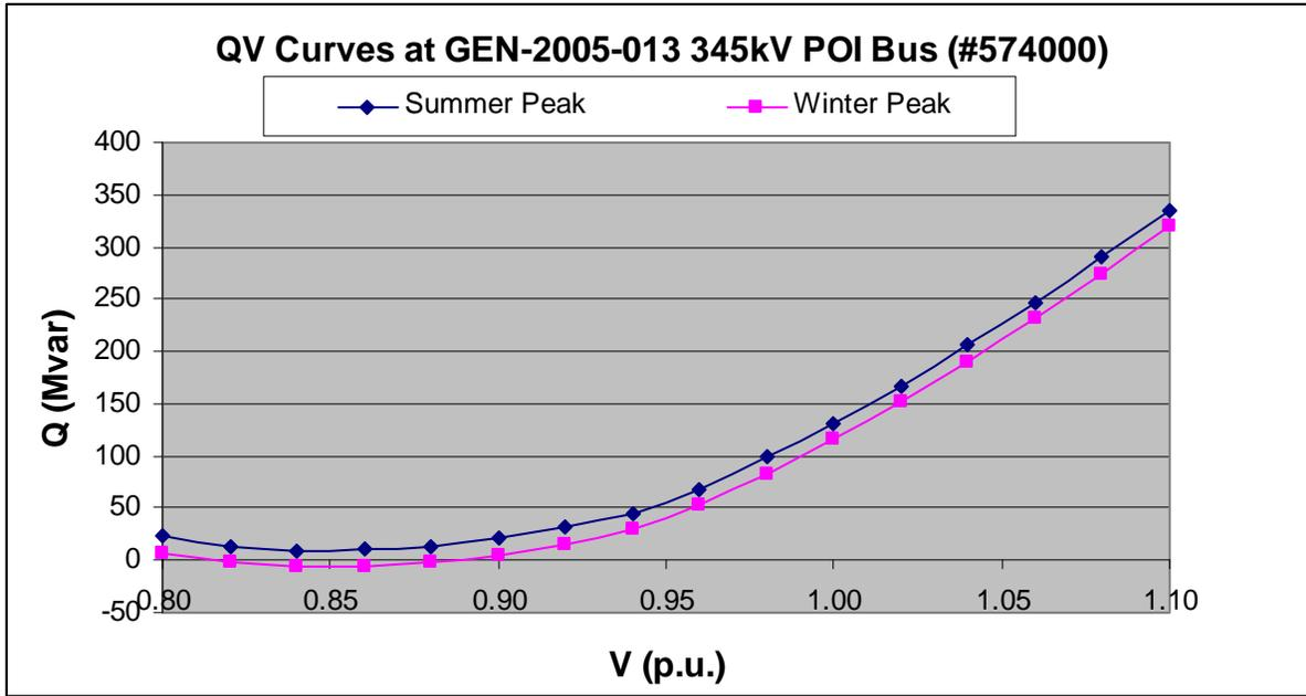
Figure 4-5. QV Curves at GEN-2005-013 345kV POI Bus with Contingency on the Rose Hill – Latham 345 kV Line
