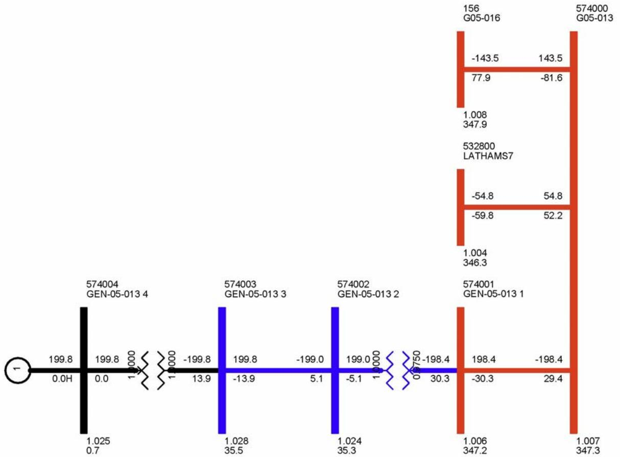
Figure 3-1. Power Flow One-line for GEN-2005-013 and adjacent equipment (SP)
